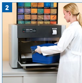
2 HF Thermal Disinfection
